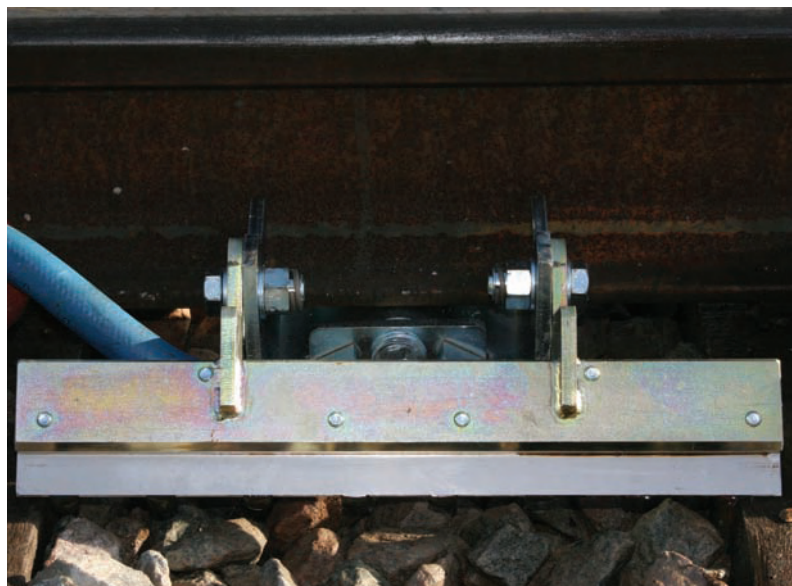
Blade dropped away for grinding
