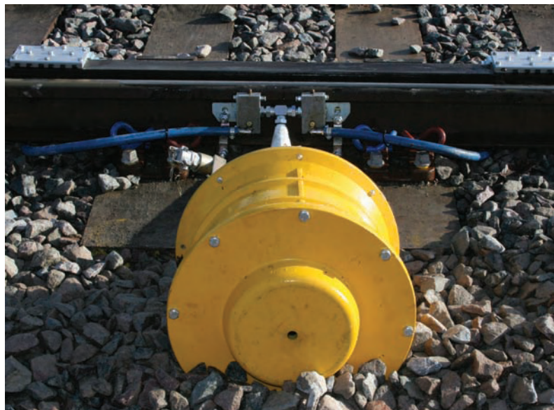
EasiCheck system on UIC33 check with Flat bottom running rail
